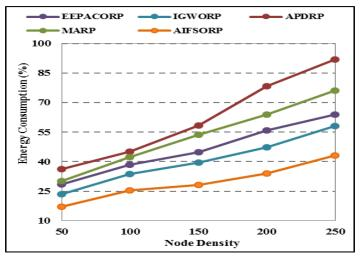
Figure 4 Energy Consumption Vs Protocols
