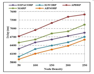
Figure 1 Packet Delay Vs Protocols
